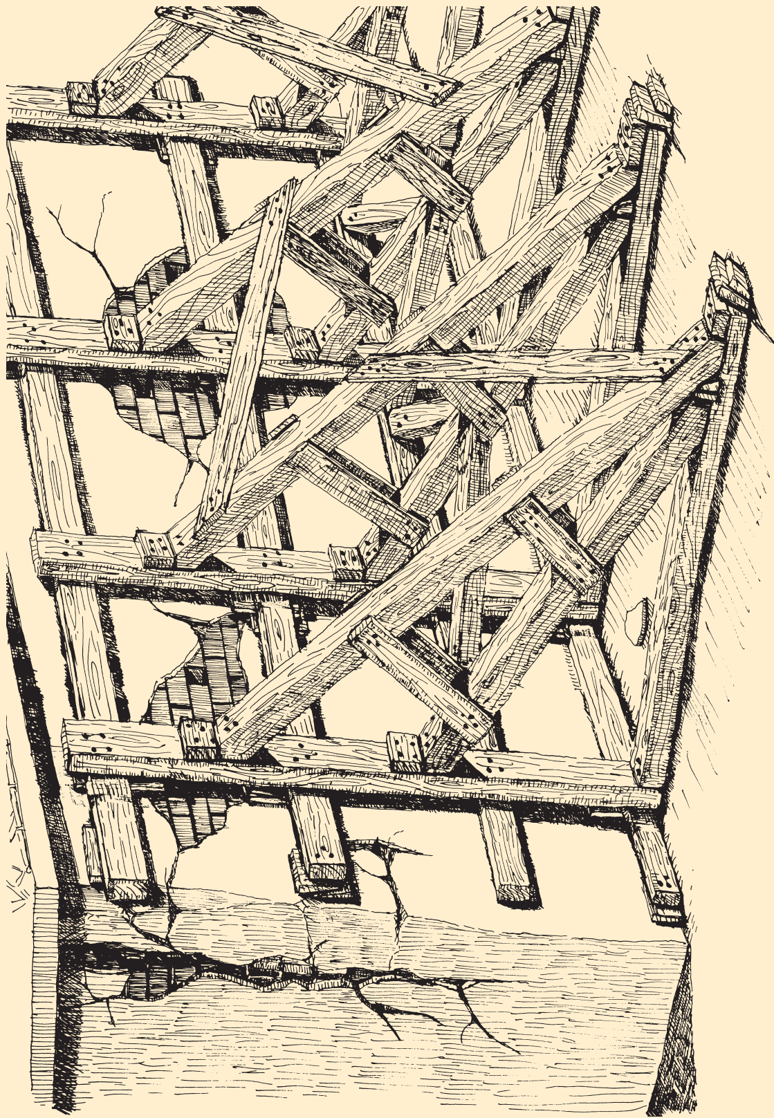
Figure 10. Extended shoring of wall using wooden raking shores.
